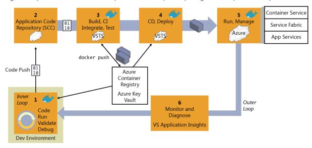
Figure 5-1: DevOps outer-loop workflow for Docker applications with Microsoft tools
