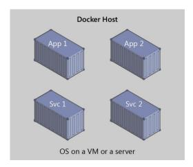
Figure 1-1: Multiple containers running on a container host
