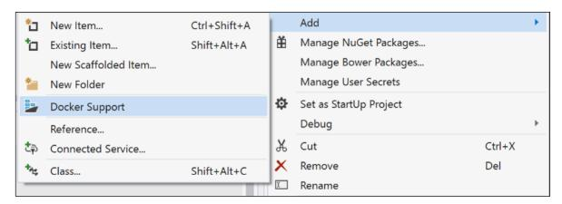
Figure 4-27: Turning on Docker Solution support in a Visual Studio 2017 project
