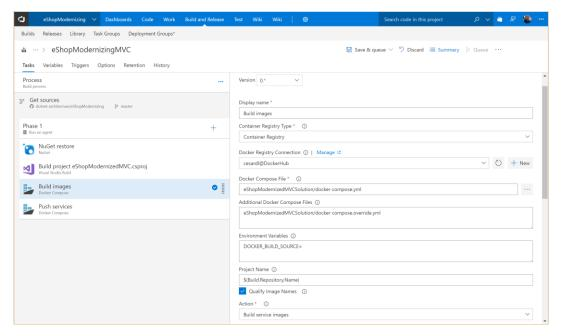
Figure 5-13: Build/CI pipeline in VSTS building Docker images and pushing images to a Docker registry
