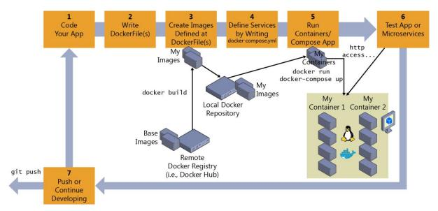
Figure 4-18: High-level workflow for the life cycle for Docker containerized applications using Docker CLI
