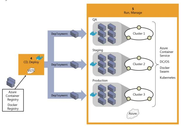
Figure 5-9: Deploying distributed applications to Container Service
