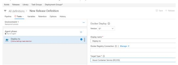
Figure 5-11: Docker Deploy task definition deploying to Azure Container Service DC/OS
