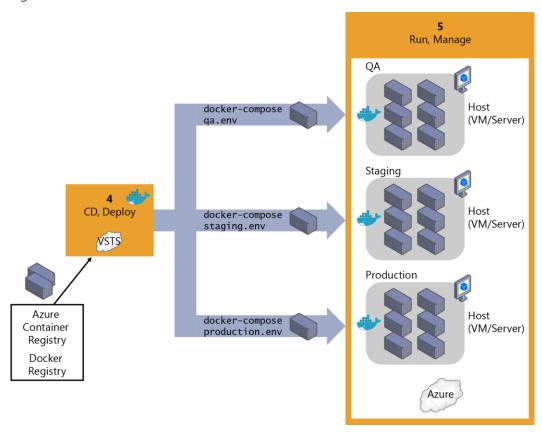
Figure 5-6: Deploying application containers to simple Docker host environments registry
