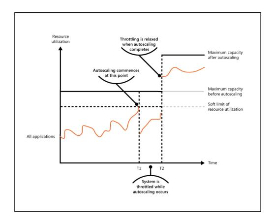
At time T1, the threshold specifying the soft limit of resource use is reached. At this point, the system can start to scale out. However, if the new resources don't become available quickly enough, then the existing resources might be exhausted and the system could fail. To prevent this from occurring, the system is temporarily throttled, as described earlier. When autoscaling has completed and the additional resources are available, throttling can be relaxed.
