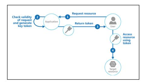
It's also possible to configure a key that has other dependencies, such as the scope of the data. For example, depending on the data store capabilities, the key can specify a complete table in a data store, or only specific rows in a table. In cloud storage systems the key can specify a container or just a specific item within a container.
